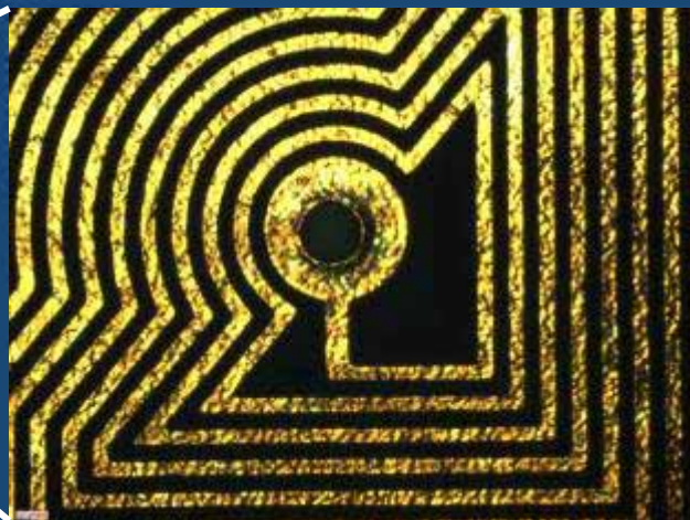
Close-up of high manufacturing complexity of HF tag
