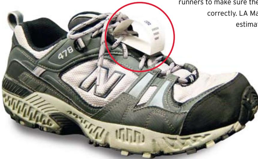
UHF Gen 2 RFID tag on a runner's shoe is an easy and inexpensive way to manage race results.
