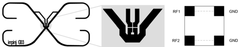
Figure 3-9 Two single-ended connections established for dual dipole antenna. Impinj Jumping Jack™ shown (L) with antenna trace detail (C) and corresponding chip/antenna connections (R).
