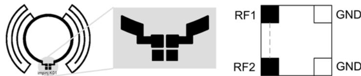
Figure 3-11 Antenna designed for differential connection. Impinj Disc™ shown (L) with antenna trace detail (C) and corresponding chip/antenna connections (R)
