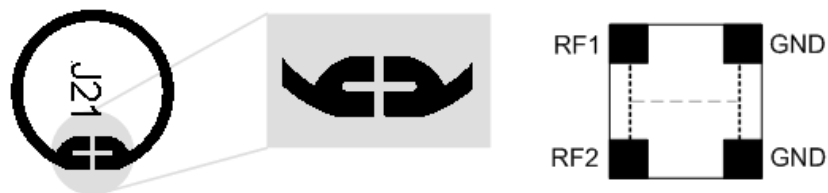
Figure 3-13 Small loop antenna (9 mm) designed for shunt connection. Impinj Button™ shown (L) with antenna trace detail (C) and corresponding chip/antenna connections (R)
