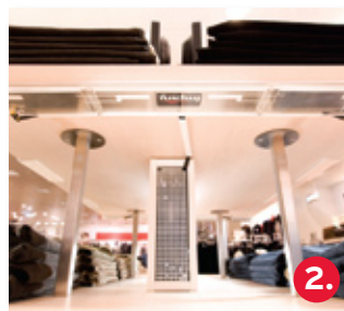
2. Impinj near-field reader antennas enable inventory monitoring, even when items are closely stacked together.
